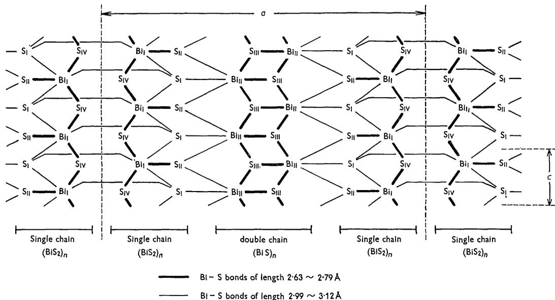
Fig. 4. Schematic representation of Bi-S bonds within a single sheet parallel to (010). Each sheet is linked to its neighbours through the Pb atoms and by bonds between Bi<sub>III</sub> and S<sub>IV</sub> (not shown).
